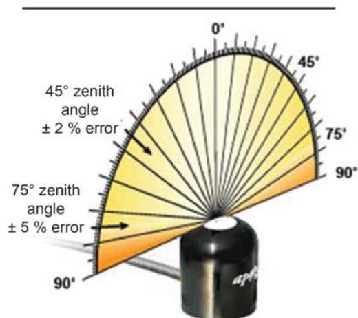
Directional, or cosine, response is defined as the measurement error at a specific angle of radiation incidence. Error for Apogee silicon-cell pyranometers is approximately  $\pm 2\%$  and  $\pm 5\%$  at solar zenith angles of  $45^\circ$  and  $75^\circ$ , respectively.
