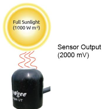
Example of total shortwave radiation measurement with an Apogee SP-212 pyranometer. Full sunlight yields total shortwave radiation on a horizontal plane at the Earth's surface of approximately 1000 W m<sup>-2</sup> s<sup>-1</sup>. This yields an output signal of 2000 mV. The signal is converted to shortwave radiation by multiplying by the calibration factor of 0.5 W m<sup>-2</sup> per mV.
