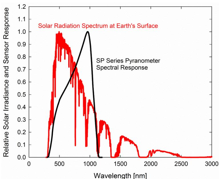
Spectral response of Apogee SP series pyranometers compared to solar radiation spectrum at Earth's surface. Silicon-cell pyranometers, such as Apogee SP series, are only sensitive to the wavelength range of approximately 350-1100 nm, and are not equally sensitive to all wavelengths within this range. As a result, when the spectral content of solar radiation is significantly different than the spectrum silicon-cell pyranometers were calibrated to, spectral errors result.
